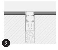
Fill surface gaps with suitable flexible sealing compound. When set remove box cover, make wiring connections and insert MOMO-F. Trim butyl liner flush if used.
