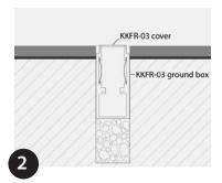
Line slot with butyl membrane if required. Drill for drainage holes in ground box and cable access hole if required. Position ground box on gravel, or permeable medium to set height to finished floor surface.
